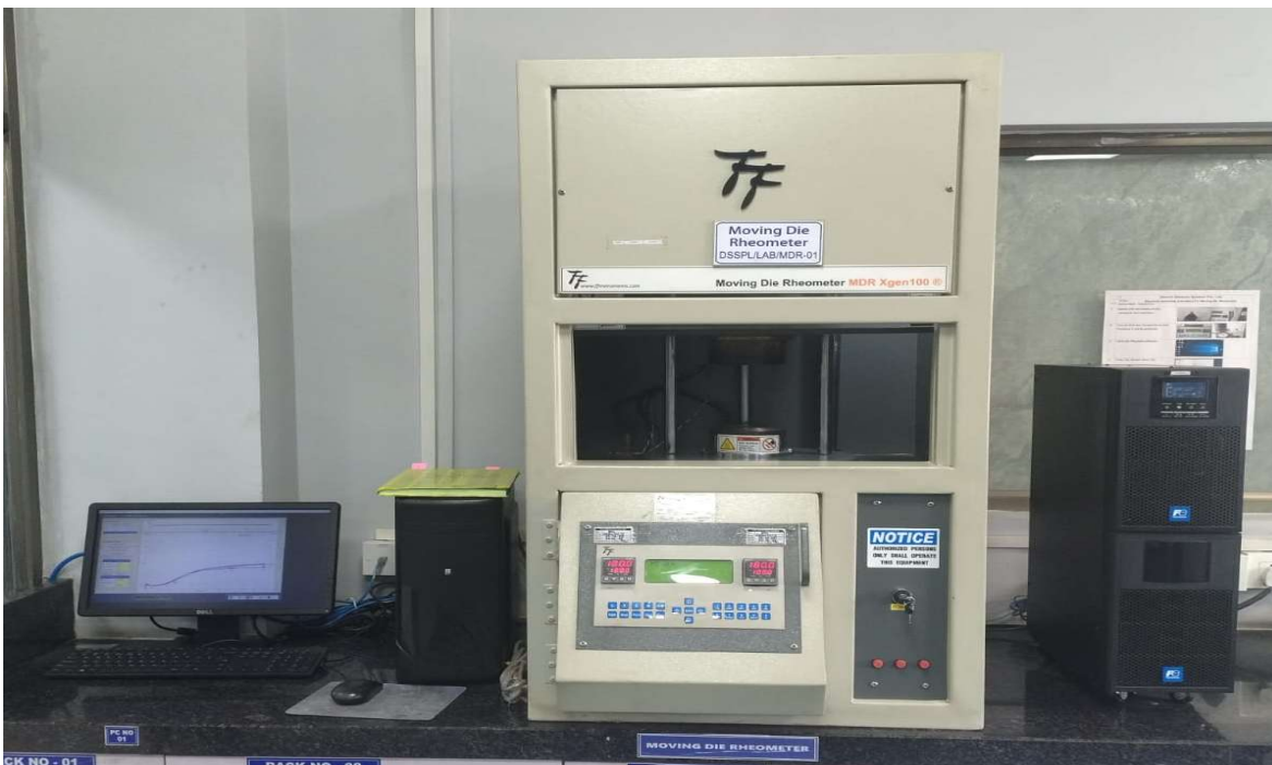
Moving Die Rheometer for Rubber Sample Testing
