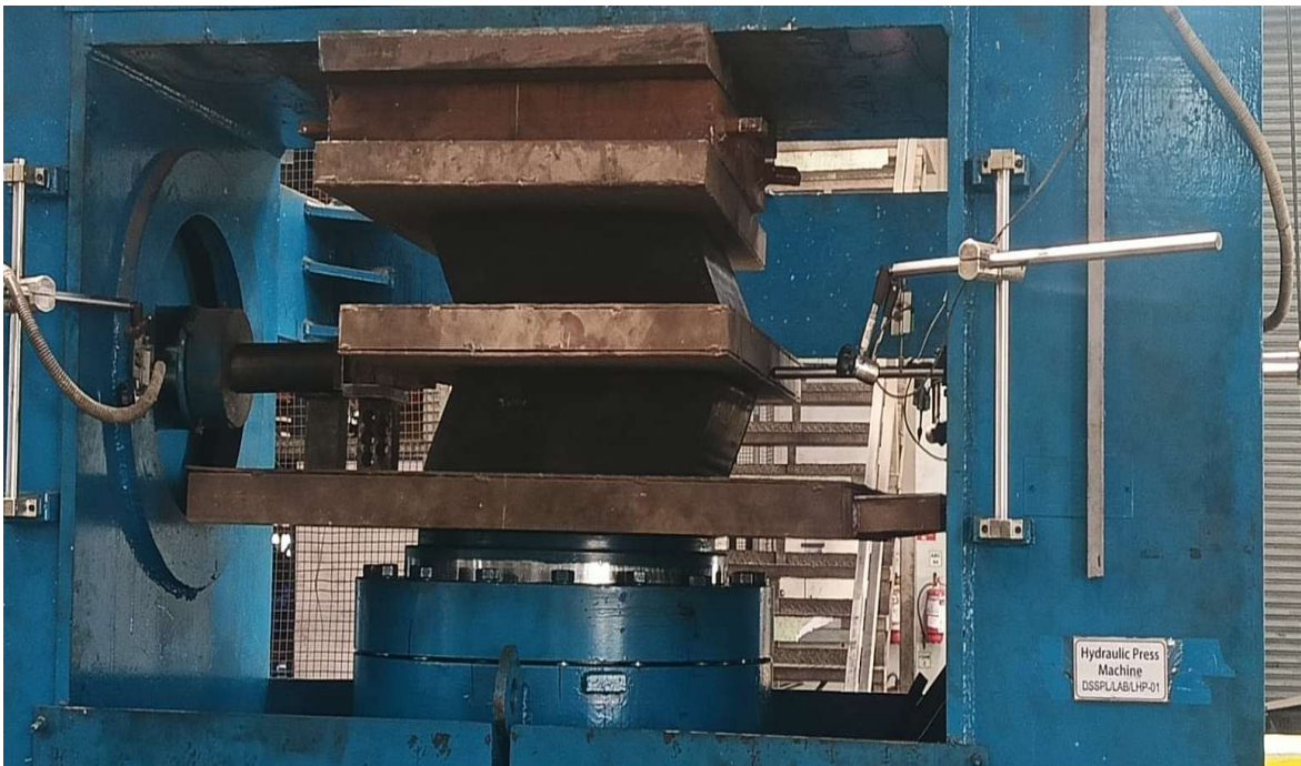
Elastomeric Bearing Shear Modules & Shear Bond Load Test Facility
