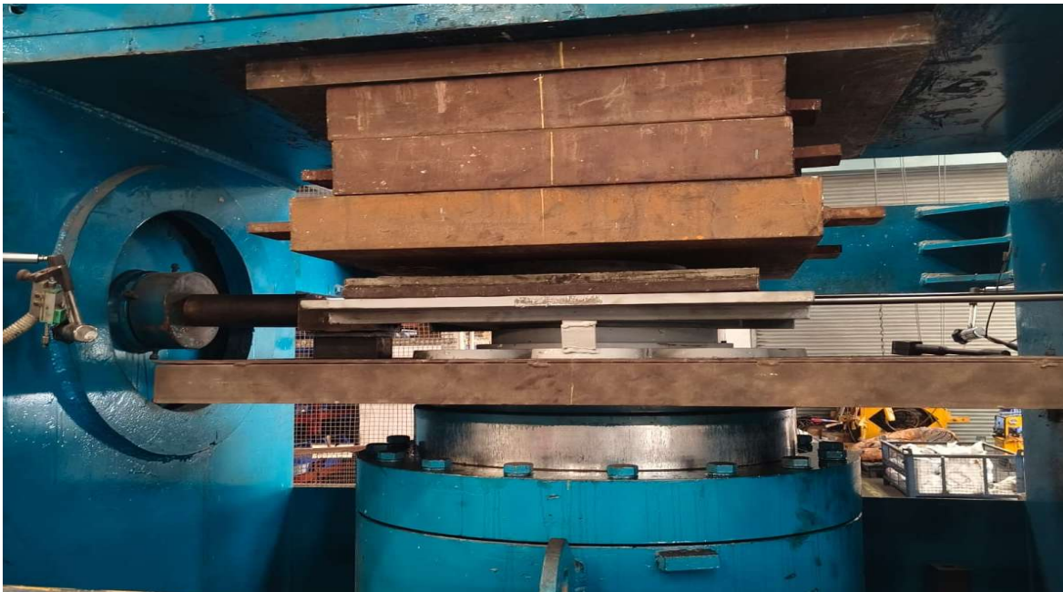
Pot Bearing Co-efficient of Friction & Combined (Vertical + Horizontal) Load Test Facility
