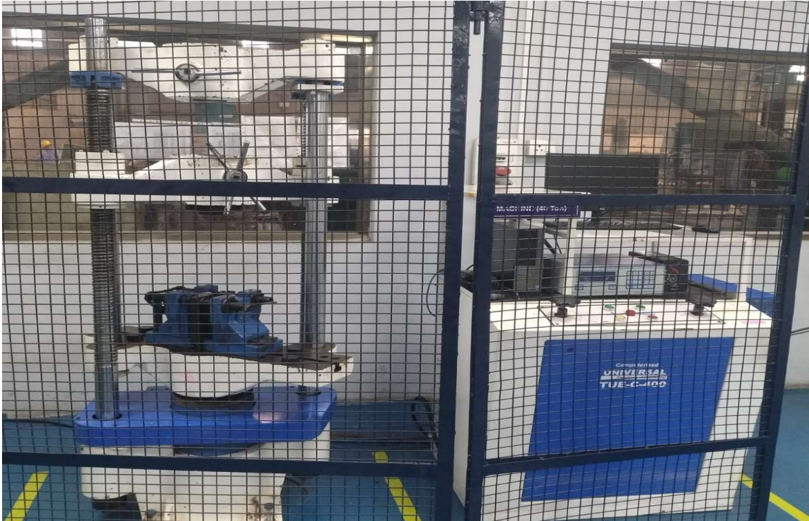
UTM for Metal Physical Properties Testing
