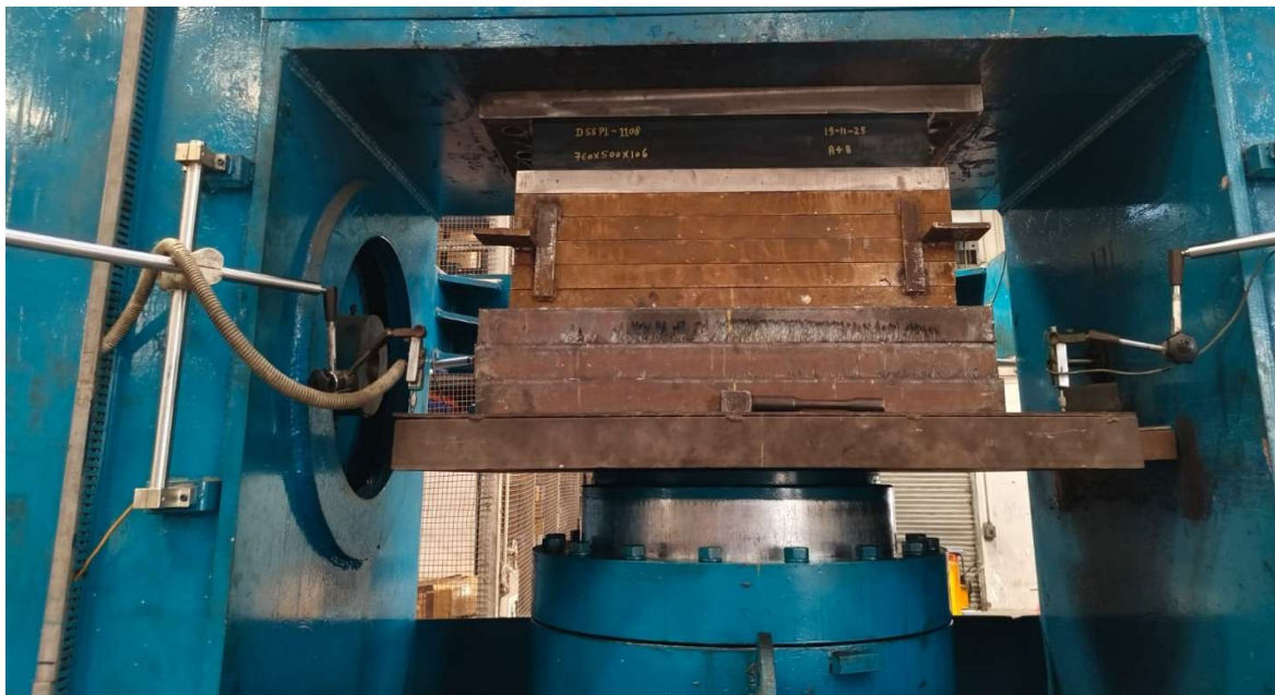
Elastomeric Bearing Axial & Compression Stiffness Load Test Facility
