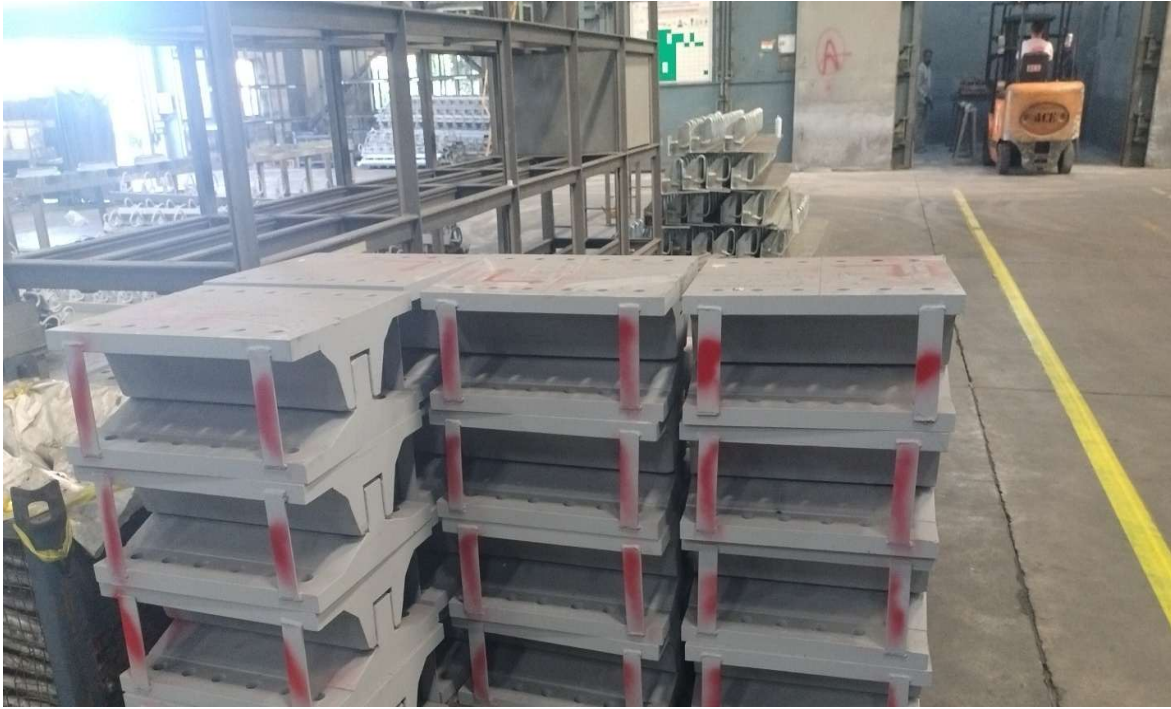
Pot Bearing Stacking Area
