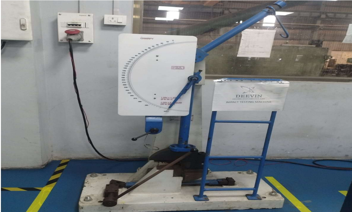
Impact Testing Machine for Metal Samples
