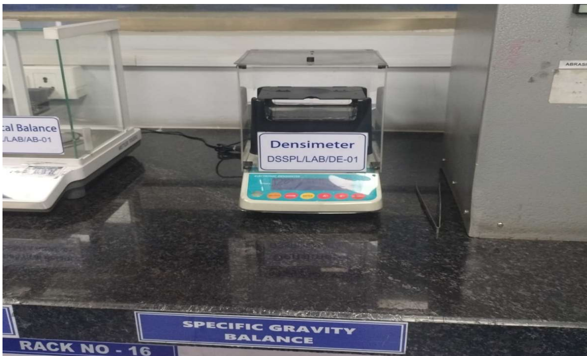
Densimeter for Specific Gravity Test
