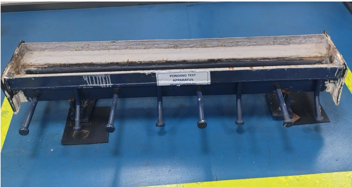
Strip Seal Expansion Joint Ponding Test Facility
