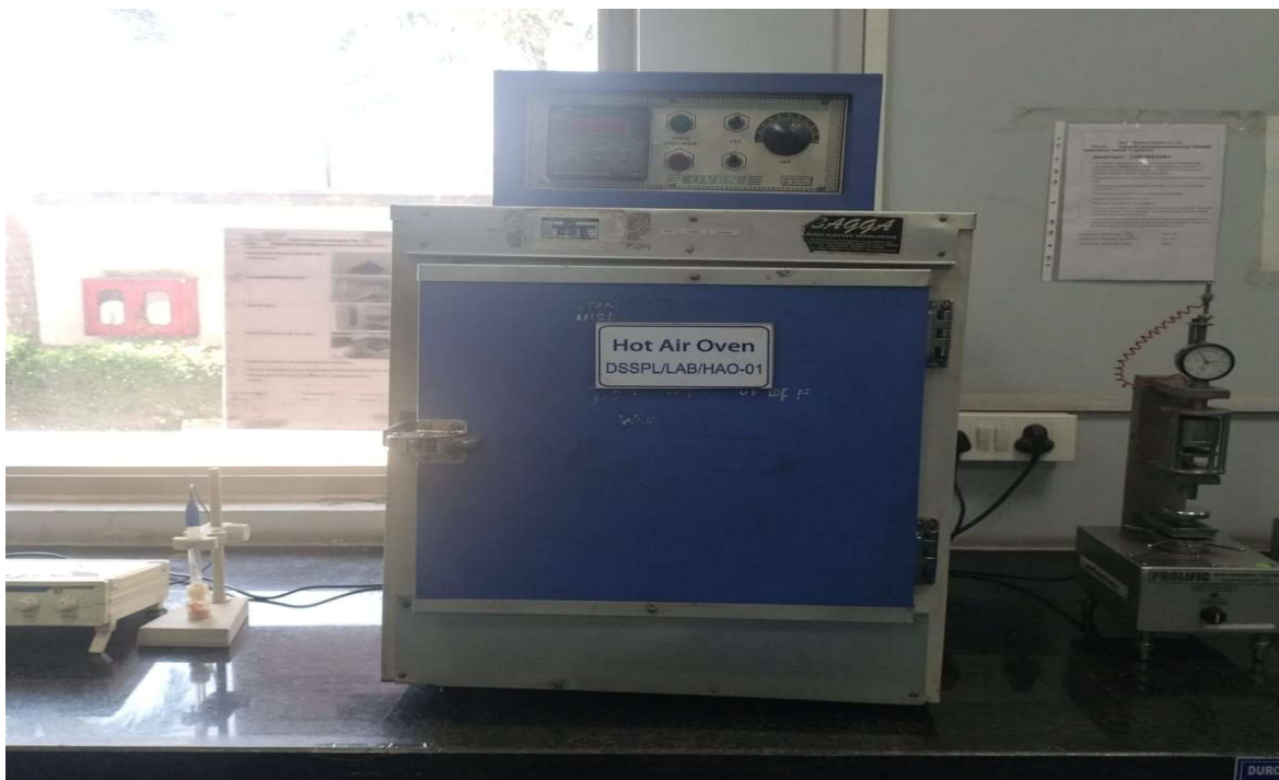
Hot Air Oven for Rubber Sample Aging Test
