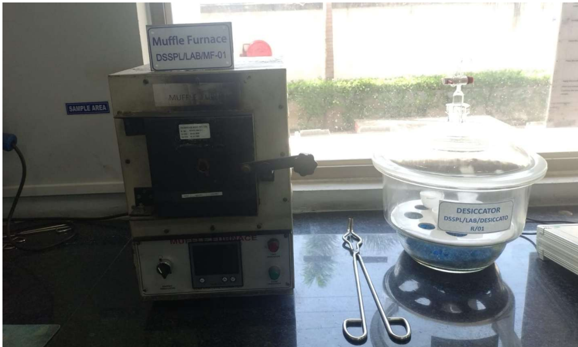
Muffle Furnace for Ash Content Test
