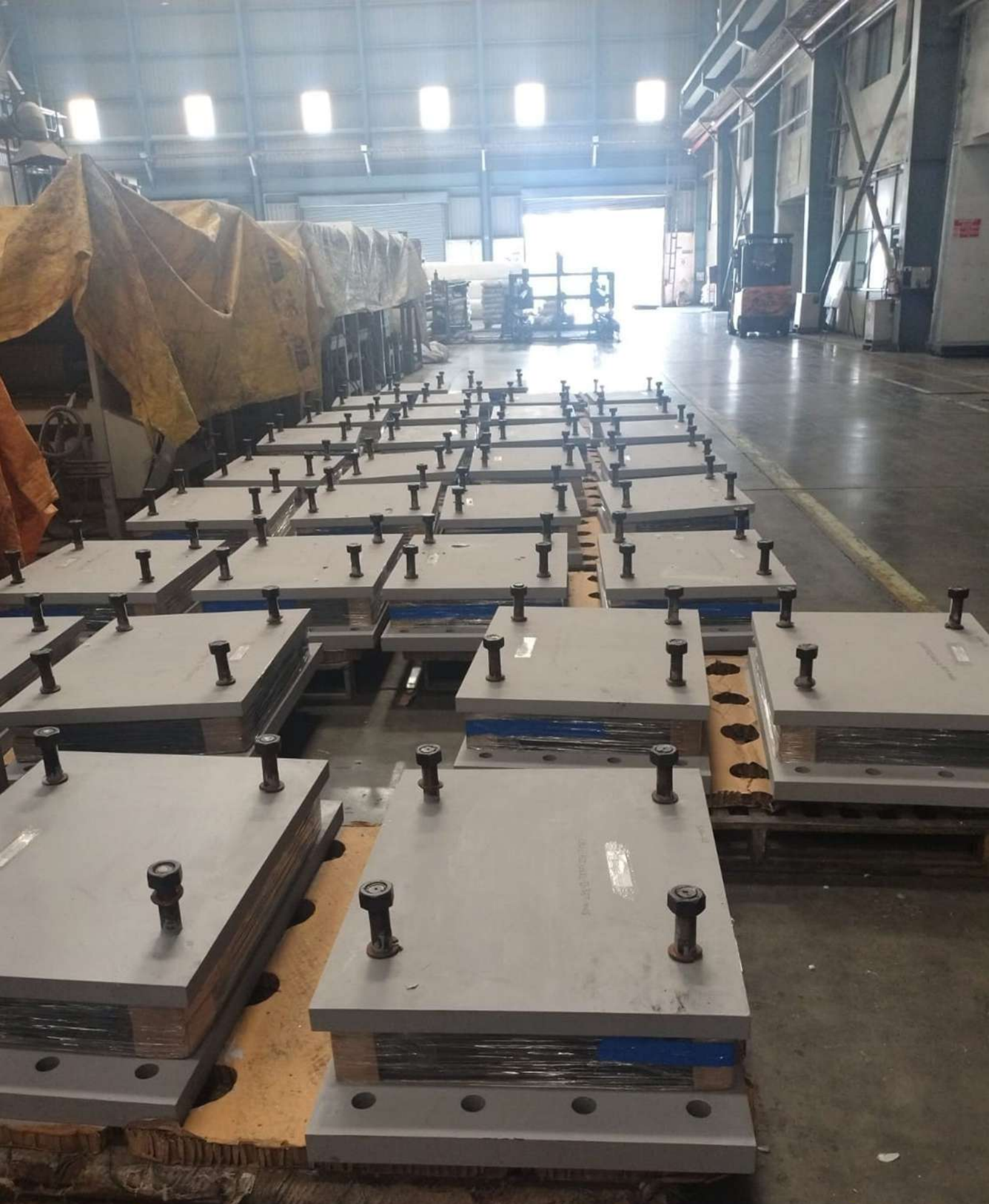
Stacking Area of Elastomeric Bearing
