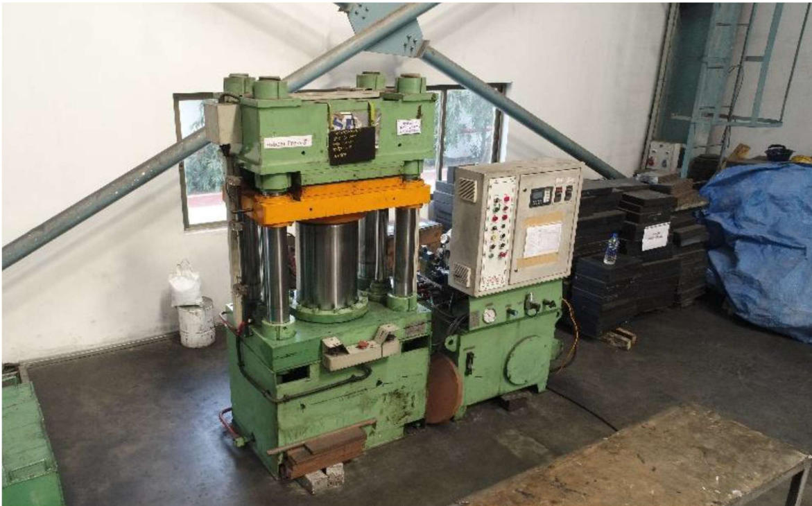
Hydraulic Press for Vulcanization of Rubber
