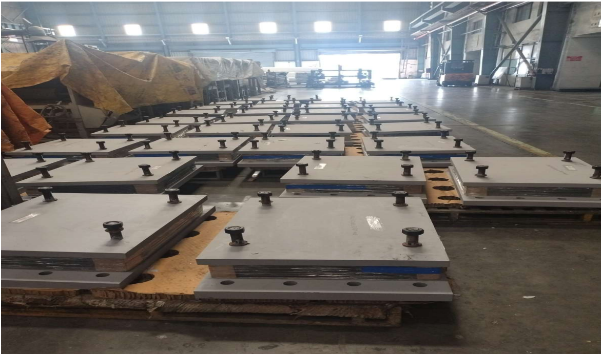
Elastomeric Bearing Stacking Area
