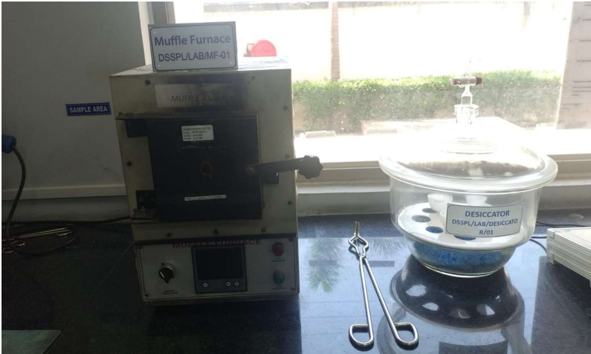
Muffle Furnace for Ash Content Test
