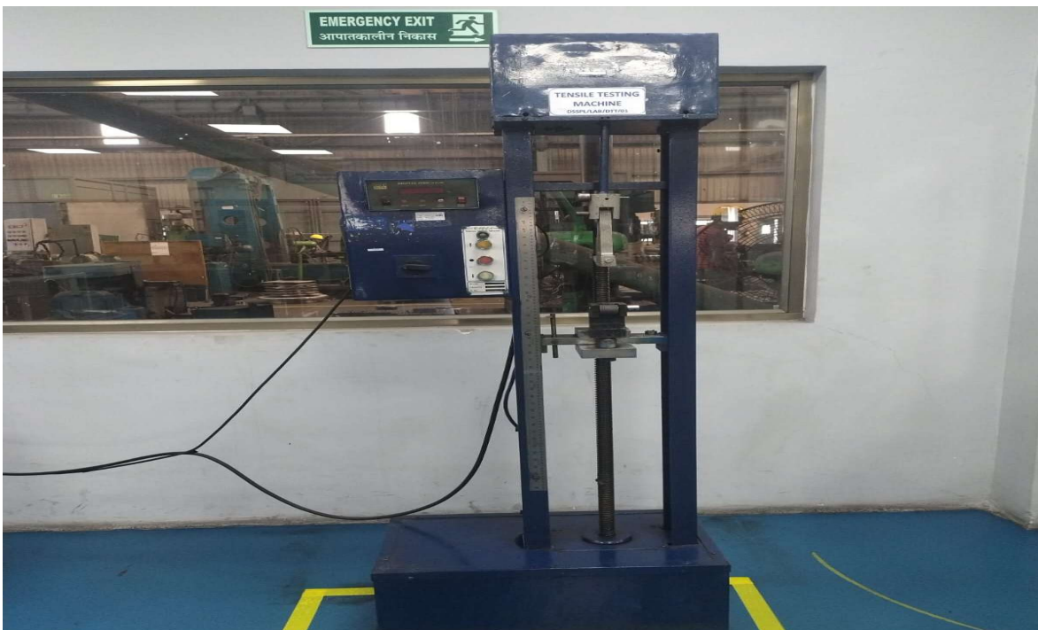
Tensile Testing Machine for Adhesive Strength & Tear Strength
