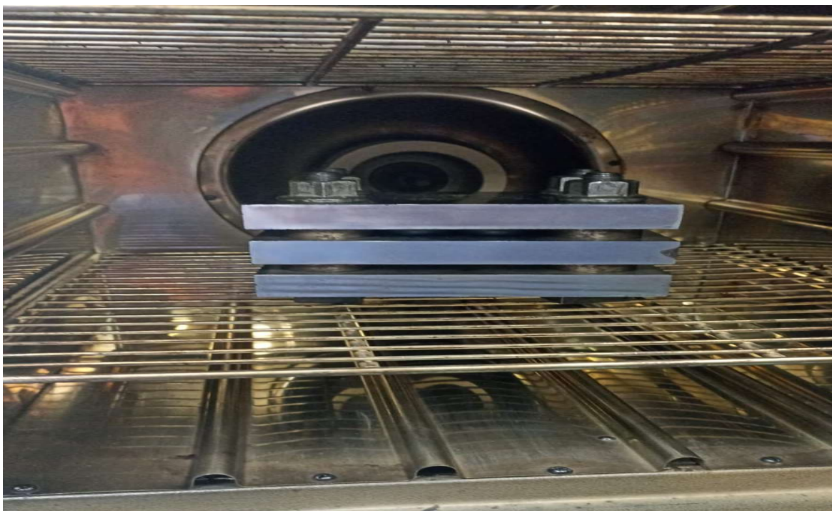
Compression Set Test Facility for Rubber Sample
