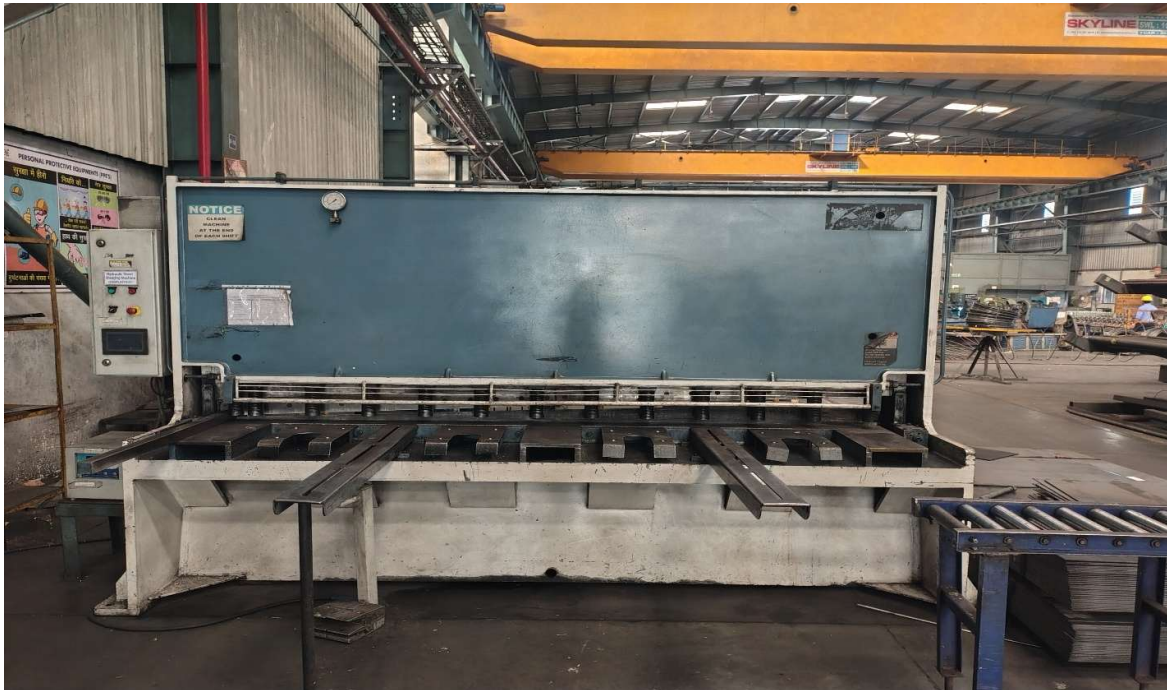
Shearing Machine for Laminates
