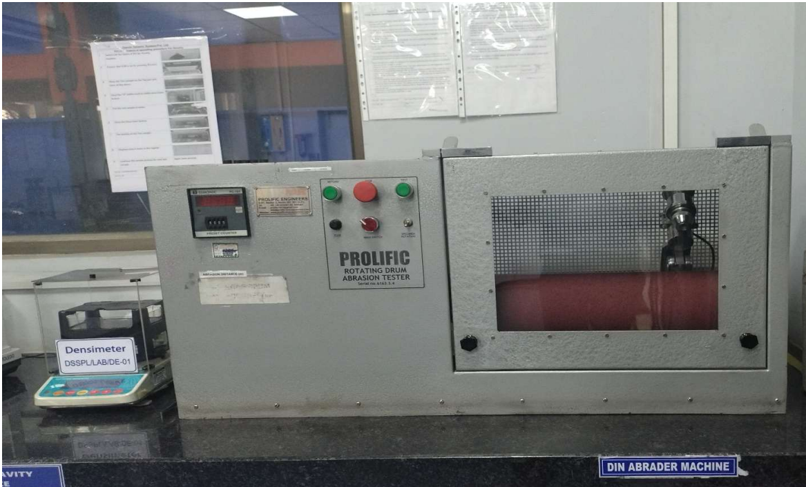
Din Abrader Machine for Rubber Sample Abrasion Test
