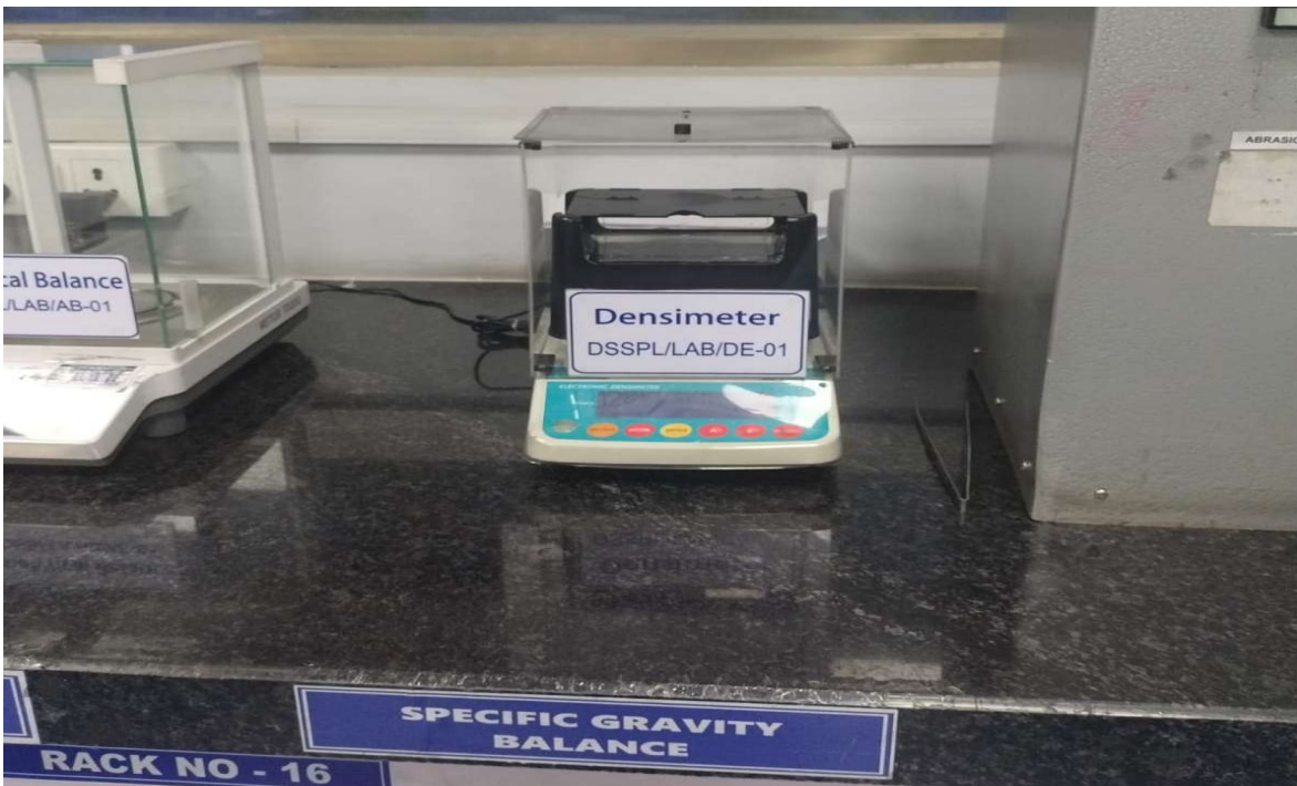
Densimeter for Specific Gravity Test
