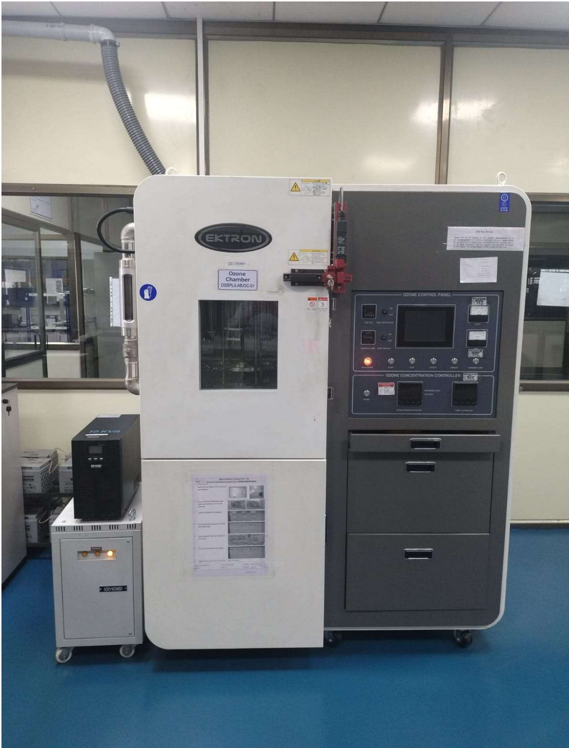
Ozone Chamber for Rubber Sample Ozone Test
