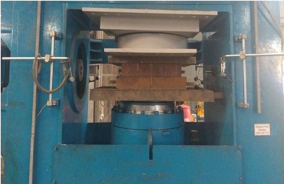
Pot Bearing Vertical & Rotation Load Test Facility
