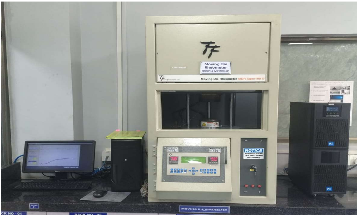
Moving Die Rheometer for Rubber Sample Testing
