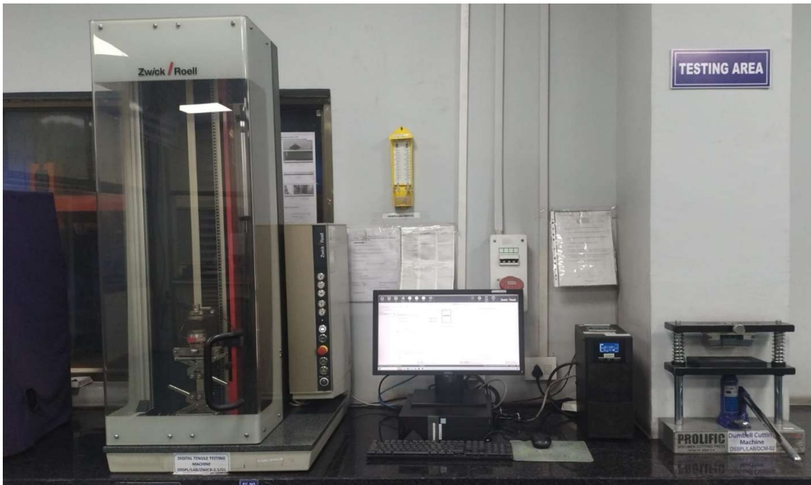
Tensile Strength & Elongation Test Facility for Rubber Samples
