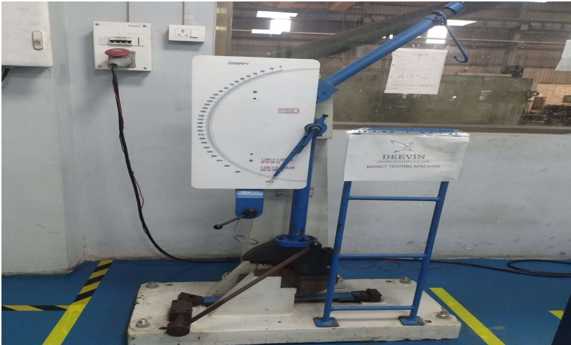
Impact Testing Machine for Metal Samples
