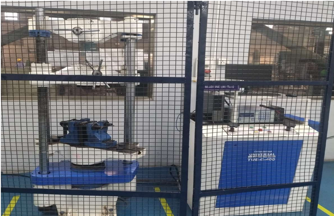
UTM for Metal Physical Properties Testing
