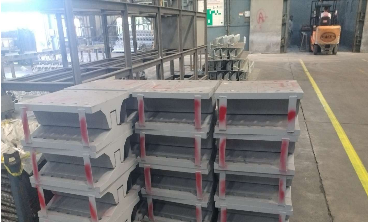
Pot Bearing Stacking Area
