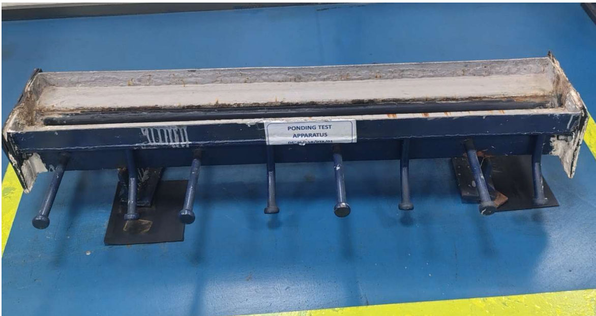
Strip Seal Expansion Joint Ponding Test Facility
